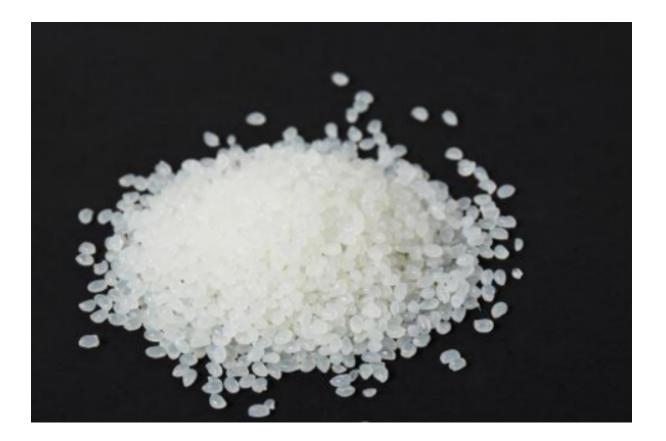
The melt index is an indicator of the fluidity of the hot melt film after melting, which affects the coatir wetting, and penetration of the adhesive on the surface of the glued material. Melt index can be close related to the hot melt adhesive process.
