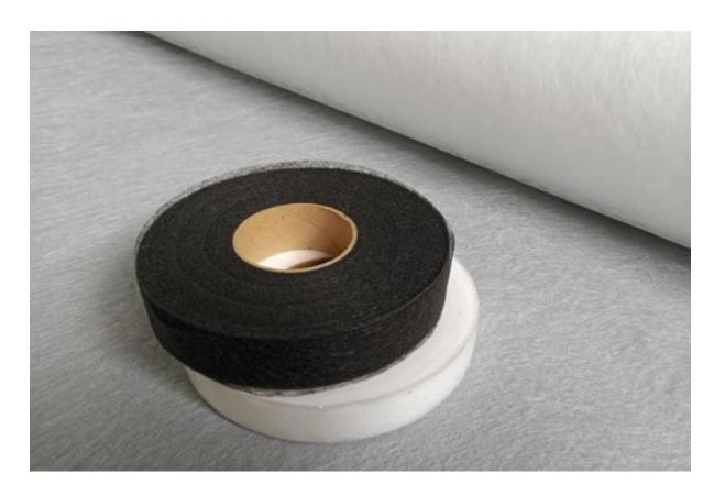
In terms of composition, hot melt adhesive film is mainly composed of polymers, such as EVA, TPU, e main component of double-sided adhesive is elastomeric resin, and there is a big difference in this re-
