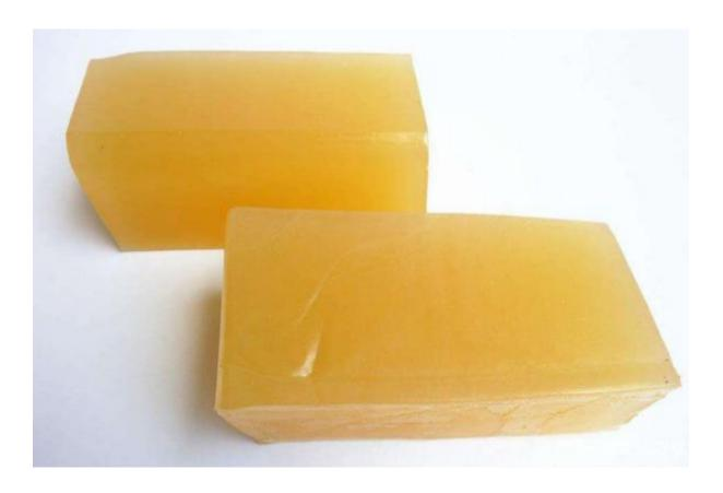
Hot melt glue blocks are also one of the forms of hot melt glue products, which are first melted in a fand then applied directly to the surface of the bonded material by a machine. Unlike hot melt glue per generally not used as a raw material for manufacturing other forms of hot melt glue products. Hot M Powder
