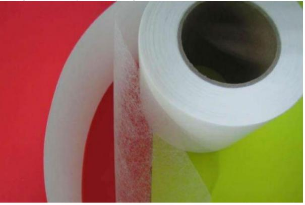
3. If the temperature of the bonded material is lower than 15 degrees, it is recommended that custor are in a position to do so should preheat the bonded material before packaging or edging operation. necessary, please add auxiliary heating facilities such as a hairdryer, heating lamps, etc., to increase temperature to achieve a good gluing effect. To ensure the quality of packaging or edge sealing.
